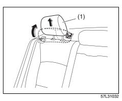
If you install the child restraint system in the rear right or left seat, remove the head restraint (1) or raise the head restraint upright and make it lock at the highest position.
